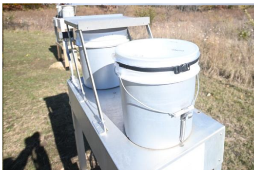
Figure 7. Seal the previous weeks sample bag bucket. Aerochem (left) and NCON (right).
