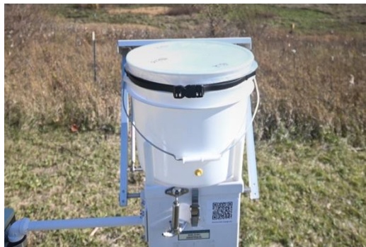
Figure 7. Seal the previous weeks sample bag bucket. Aerochem (left) and NCON (right).
