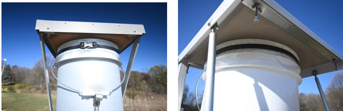
Figure 13. Check the lid pad seal on the sample bag bucket. Aerochem (left) and NCON (right).
