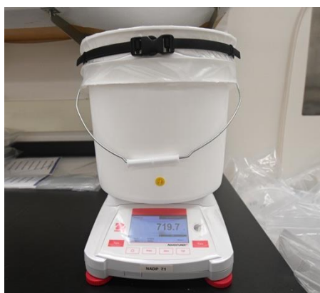
Figure 9. Weigh NTN bucket, sample bag, bucket strap, bucket plug, and lid
