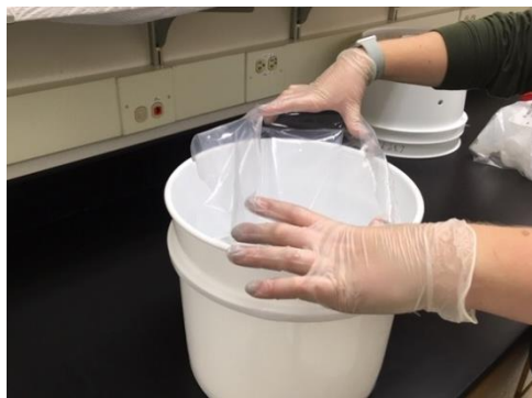
Figure 3. Open the sample bag starting at the top of the bag.
