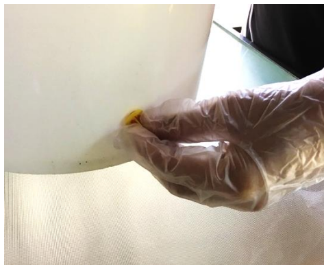
Figure 7. Insert bucket plug in the hole on side of NTN bucket to prevent water from entering.
