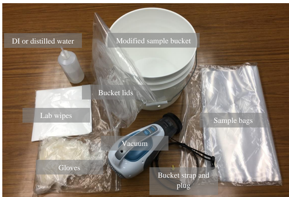
Figure 1. Items needed to deploy sampling bag.
