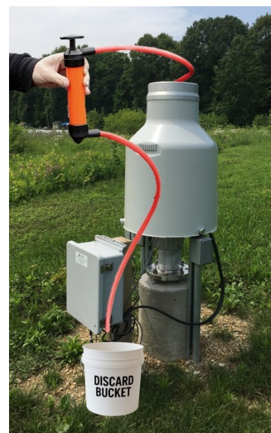
Figure 2. Transfer pump with OTT Pluvio
