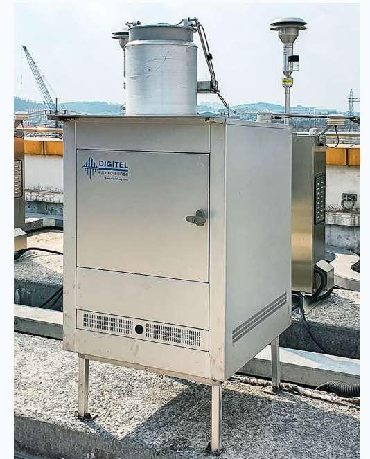
Reference photo of a DRA-12 installed on a concrete slab
