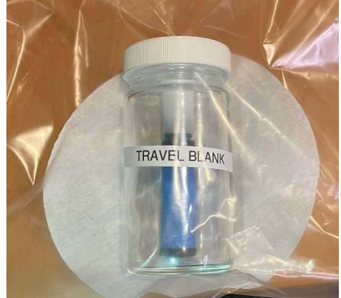
Figure 7. Travel Blank with citric acid filter paper. (leave in sealed jar in shipping box).
