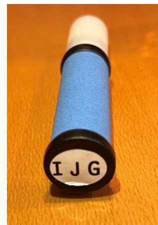
Figure 1. Radiello passive sampler with 3 character body ID.
