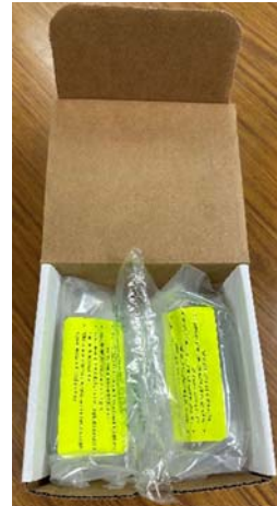
Figure 3. Supply box with one or duplicate sampler(s) and a Travel Blank.
