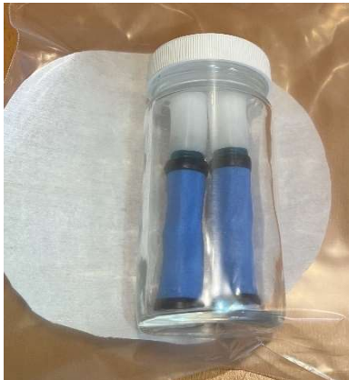
Figure 5. Two samplers to deploy with citric acid filter paper.
