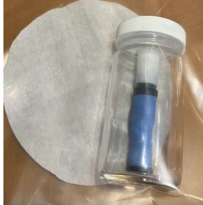
Figure 6. One sampler to deploy with citric acid filter paper.
