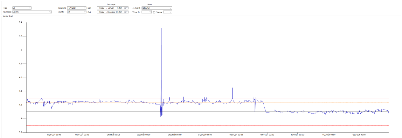
Figure 35. pH low-level (FL) standard recoveries. The outlier was due to issues during calibration of the probe which were resolved within that run day. There is a slight high bias until 8/30/2021 when a new stock of the reagent was received.
