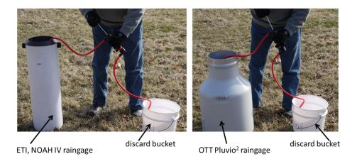
3. If the raingage is winterized, place the other end of the "discharge" tubing in a discard bucket or other container to collect the anti-freeze/water mixture. If the raingage is not
