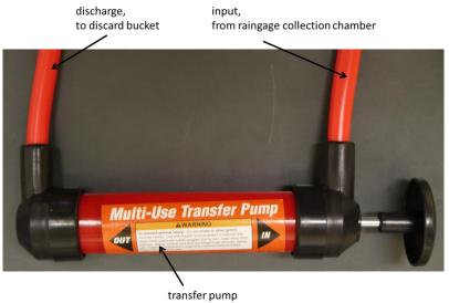
2. Place the other end of the "input" tubing in the collection chamber of the raingage.
