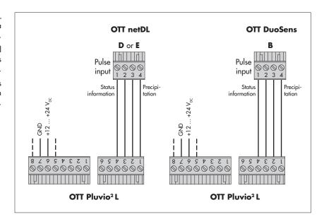
Fig. A5: Connecting the OTT Pluvio<sup>2</sup> L to an OTT netDL or OTT DuoSens via the pulse output.
