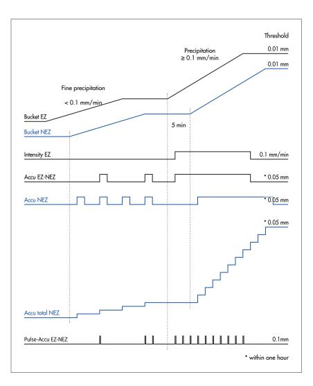
Fig. 3: Schematic display of measured value output for different precipitation values of the OTT Pluvio2 L for fine precipitation (< 0.1 mm/min) and precipitation (≥ 0.1 mm/min).
