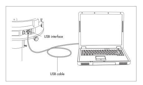
Fig. 21: Connecting the OTT Pluvio<sup>2</sup> L to the PC using the USB interface.
