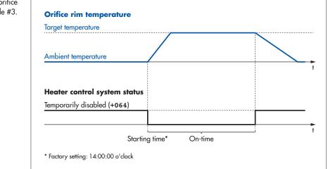
Mode #4 Heater control system is operated based on precipitation events. Once precipitation has started, the heater control will be active for a preset after-run time (1 ... 1440 minutes) and continuously keep the orifice rim temperature at the predetermined setpoint. Outside this after-run time, the heater self-test is performed based on a selectable interval (1 h ... 7 d).
