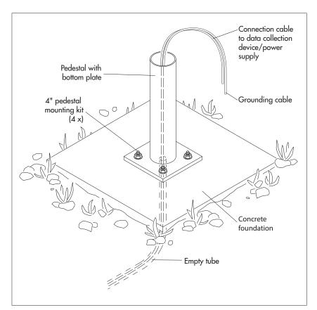
Fig. 7: The location prepared for installing the OTT Pluvio<sup>2</sup> L.
