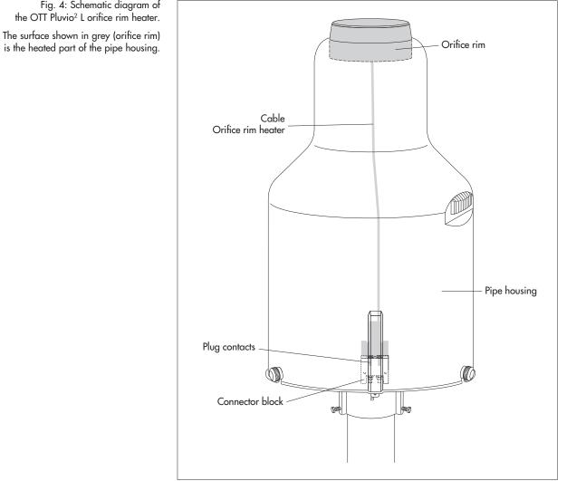
Fig. 4: Schematic diagram of the OTT Pluvio<sup>2</sup> L orifice rim heater.
