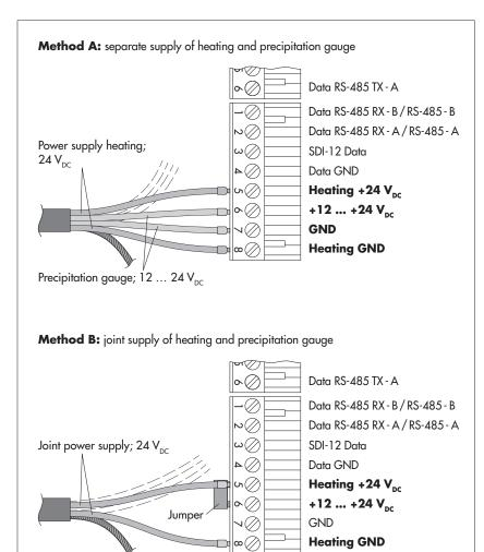
Fig. 11: OTT Pluvio<sup>2</sup> L with orifice rim heater: Connecting options for power supply of the precipitation gauge and orifice rim heater.
