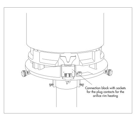
Abb. 19: Connection block for the plug contacts for the orifice rim heater.
