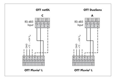
Fig. A1: Connecting the OTT Pluvio<sup>2</sup> L to an OTT netDL or OTT DuoSens via the SDI-12 interface.
