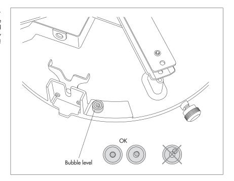
Fig. 15: Levelling the OTT Pluvio<sup>2</sup> L unit.
