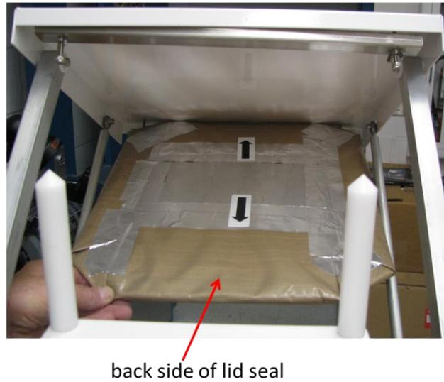
4. Remove old lid seal and set aside for return to the Network Equipment Depot (NED).
