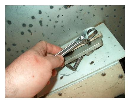
4. Remove the screws (4) that secure the motorbox to the top of the collector (see arrows in the image below). Remove the dry-side bucket to access the 4<sup>th</sup> screw. It is located inside the bucket holder under the dry-side bucket.
