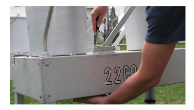
10. Using hardware from step 4, attach the clutch arm bolt to the push rod and the motorbox. Do not over tighten the bolt.
