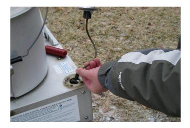
5. Note the slot in the connector attached to the sensor cable. Align the sensor connector with the corresponding motorbox connector. Tighten the connector to the motorbox.
