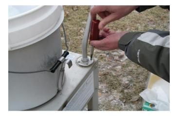
3. Remove the old sensor and set aside for return to the NADP Network Equipment Depot (NED).
