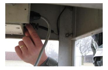
2. Unscrew the four screws securing the sensor to the frame of the collector. Be careful not to drop or misplace the screws as they will be re-used with the replacement sensor.
