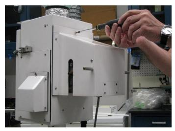
10. Disconnect the power cable connecting the motorbox to the collector.
