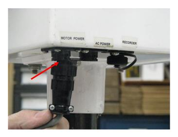
11. Remove the nuts that secure the motorbox to the back of the collector. Hold the motorbox in place when removing the last nut so the motorbox does not fall to the ground. Again, be careful not to drop or misplace the nuts. They will be used when reassembling the collector.
