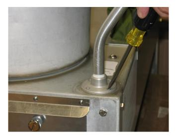
3. Remove the old sensor and set aside for return to the NADP Network Equipment Depot (NED).
