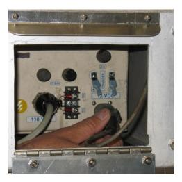
2. Unscrew the four screws securing the sensor to the frame of the collector. Be careful not to drop or misplace the screws as they will be re-used with the replacement sensor.
