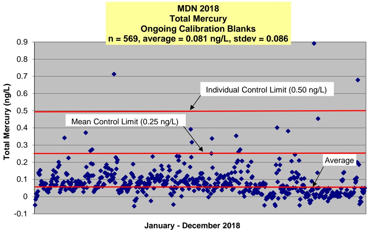
**Figure 7 - Total Mercury Continuing Calibration Blanks, 2018**
