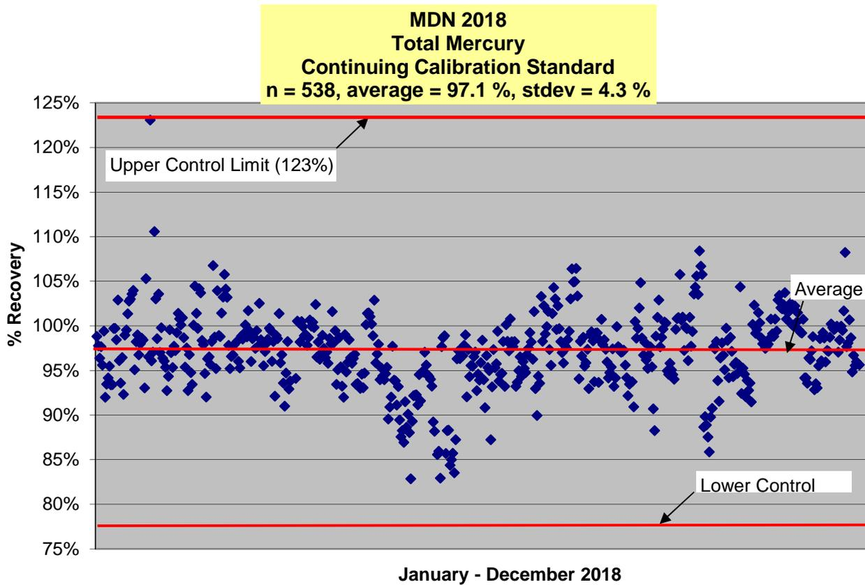
**Figure 5 - Total Mercury Continuing Calibration Standard Percent Recovery, 2018**
