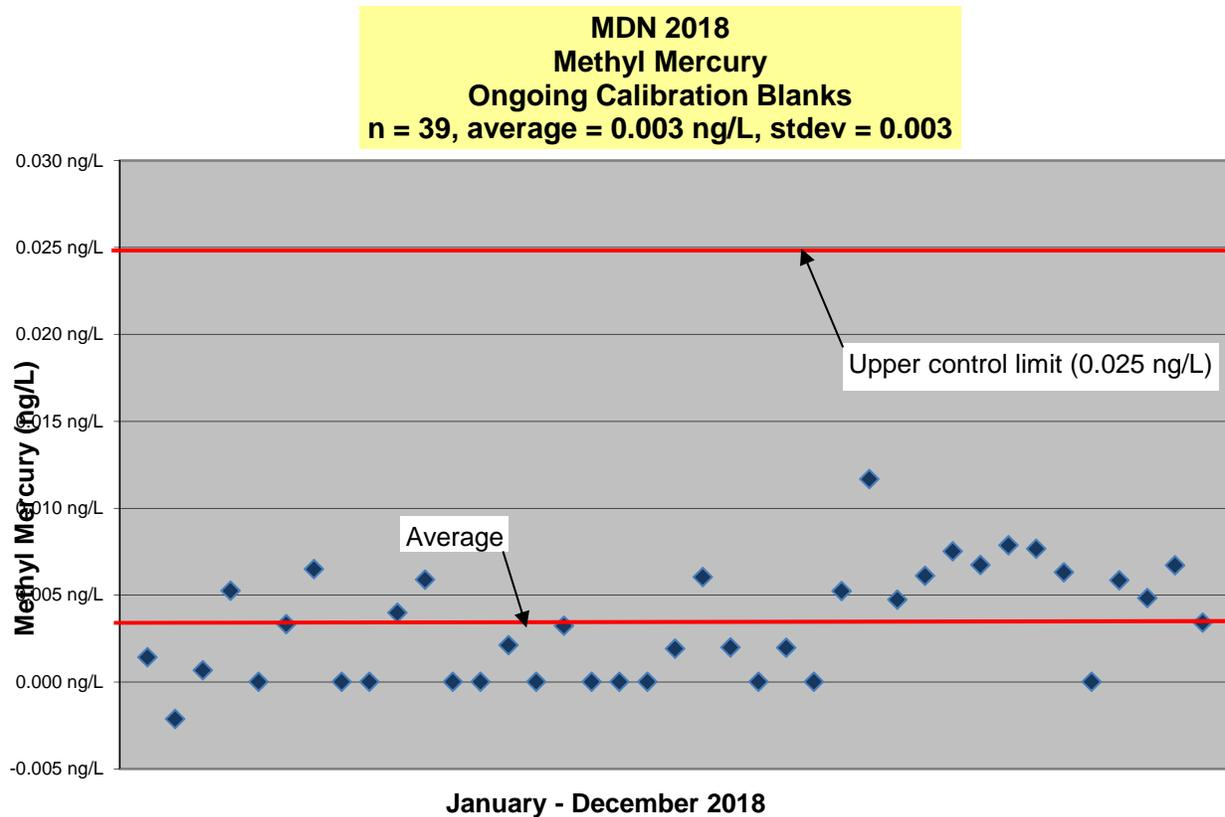
**Figure 8 - Methyl Mercury Continuing Calibration Blanks, 2018**
