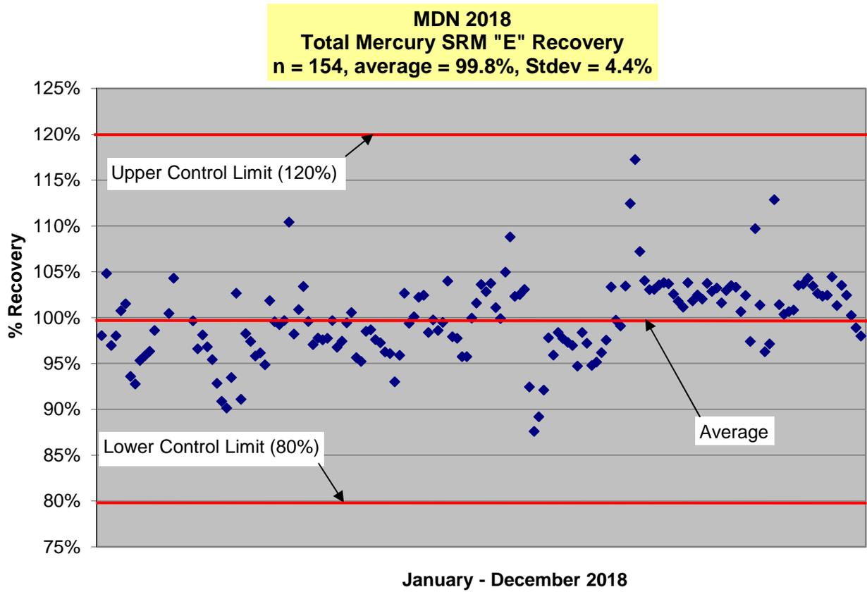
**Figure 14 - Total Mercury Percent Recovery in Certified Reference Material Samples, 2018**
