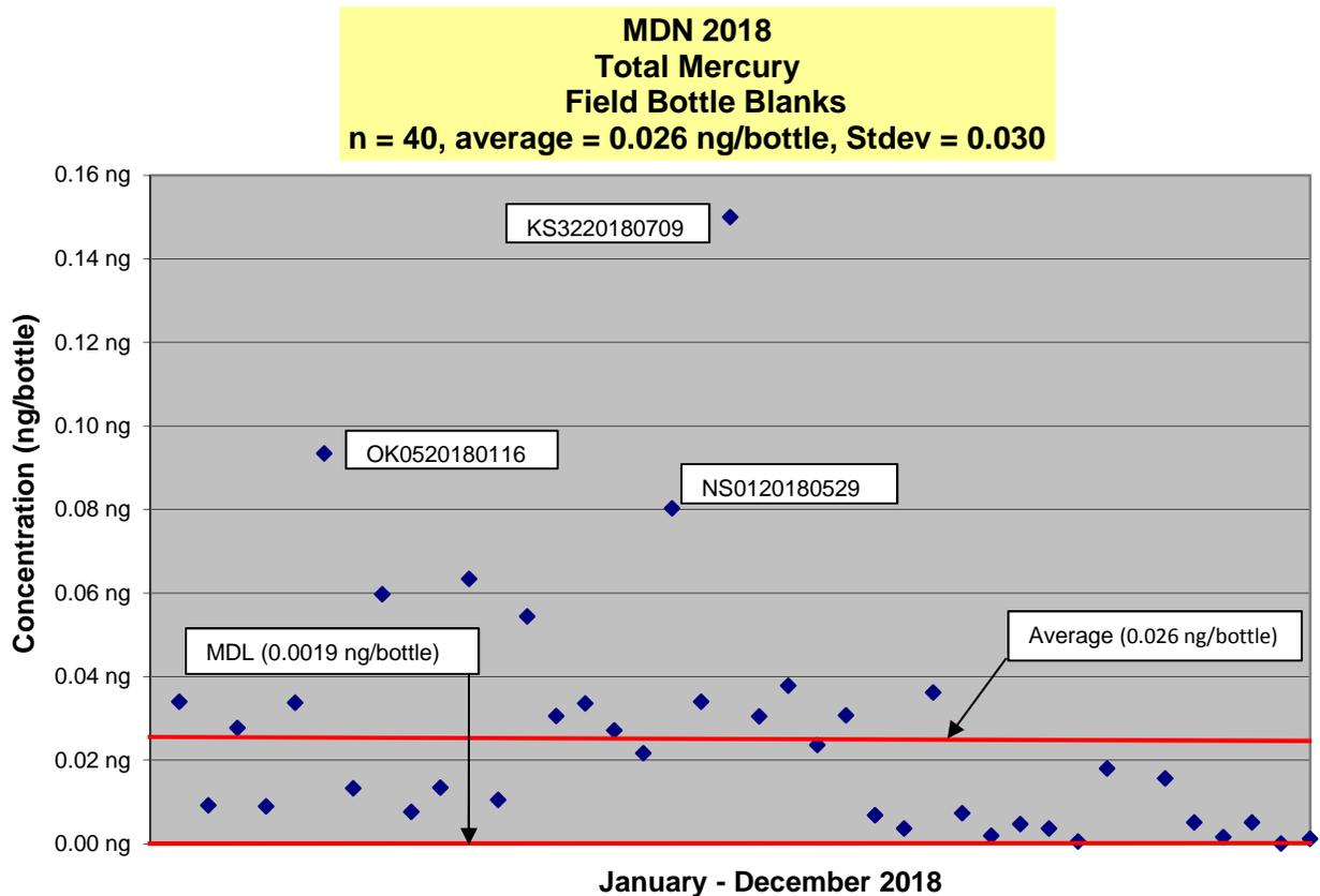
**Figure 19 - Total Mercury Concentrations in Field Bottle Blanks, 2018**
