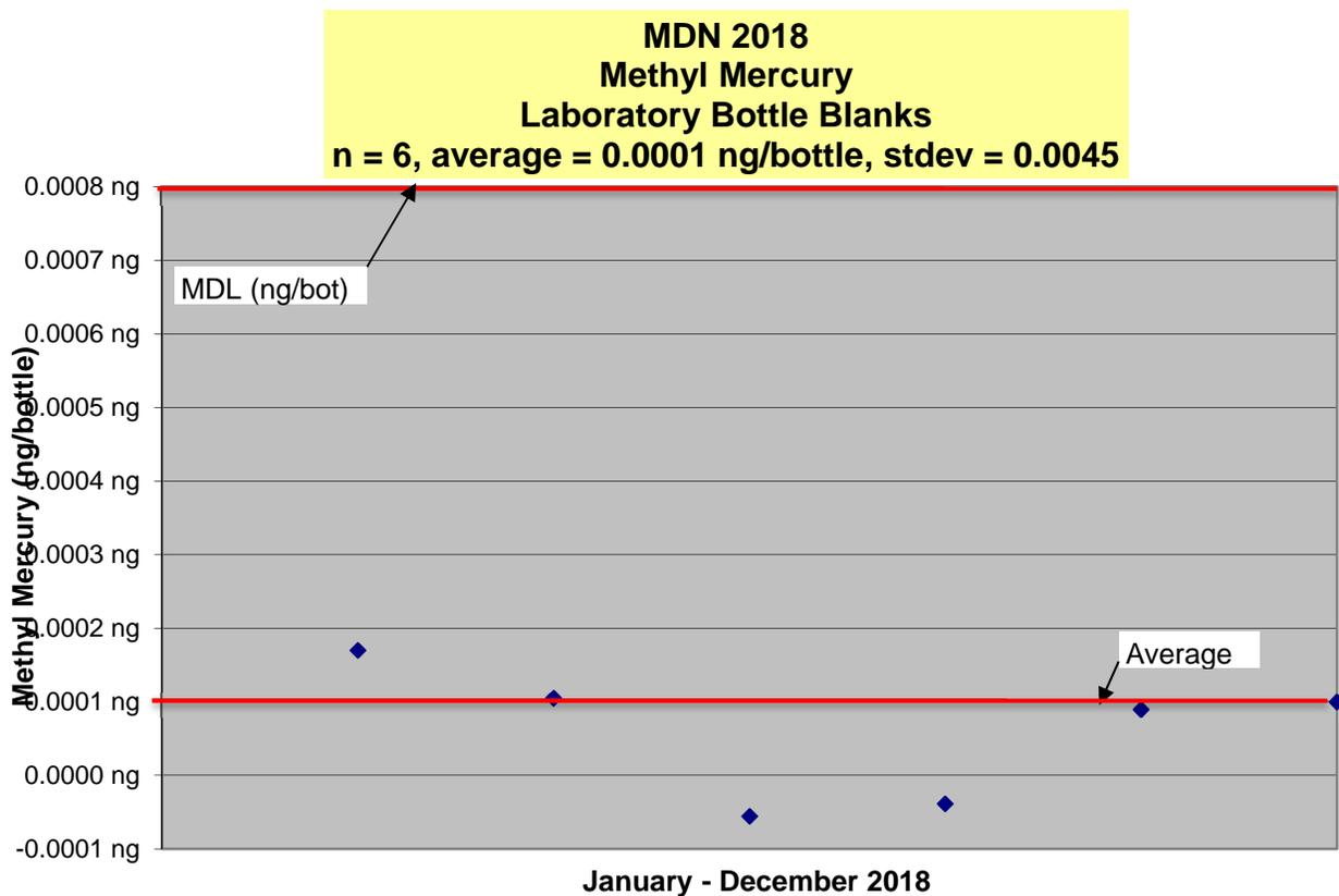
**Figure 2 - Methyl Mercury Mass in Laboratory Bottle Blanks for 6 Samples, 2018**
