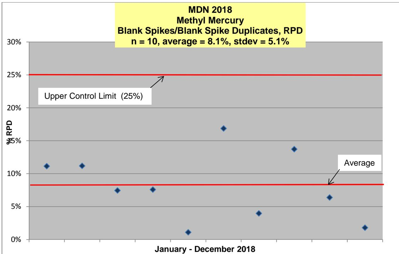
**Figure 17 - Methyl Mercury Relative Percent Difference (RPD) in Blank Spikes/Blank Spike Duplicate Samples, 2018**
