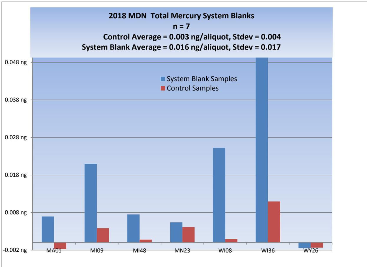
**Figure 20 - Total Mercury Concentration Data for USGS System Blanks and Control Samples During 2018**
