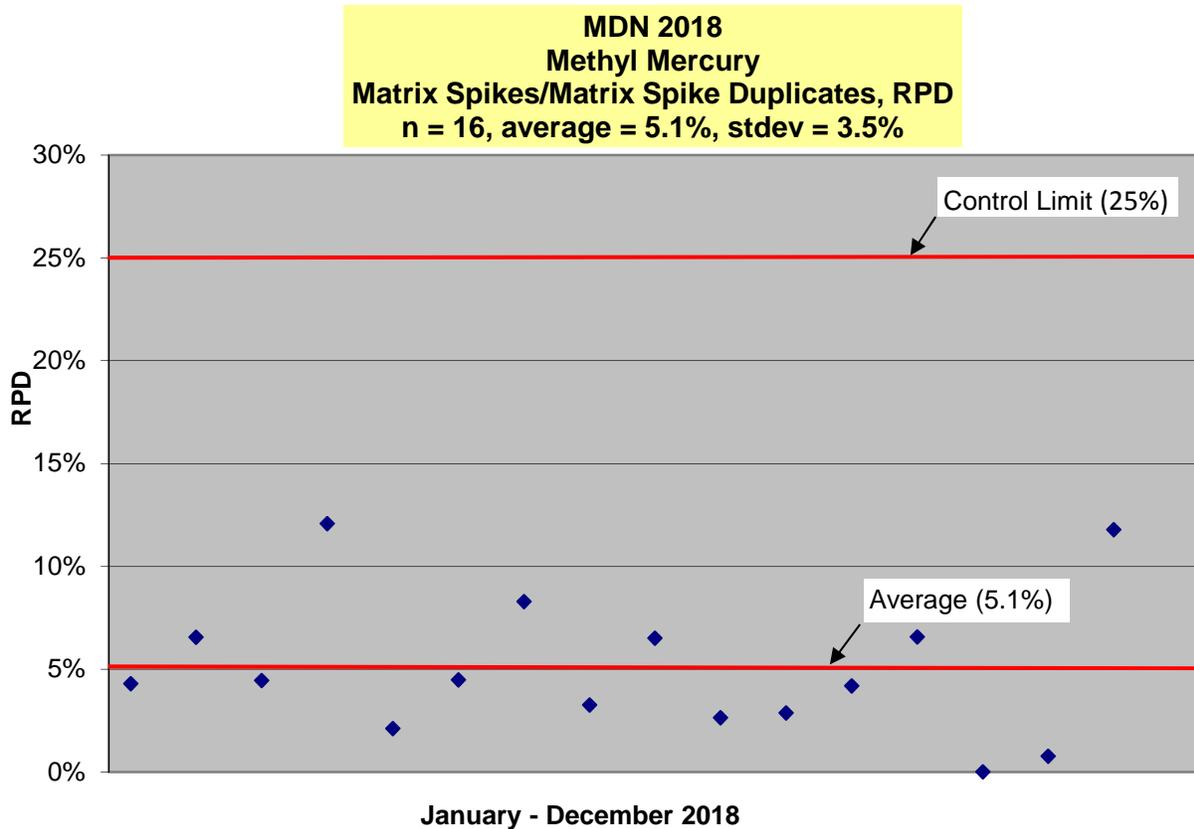
**Figure 13 - Relative Percent Differences (RPD) for Methyl Mercury Matrix Spike/Matrix Spike Duplicate Pairs, 2018.**
