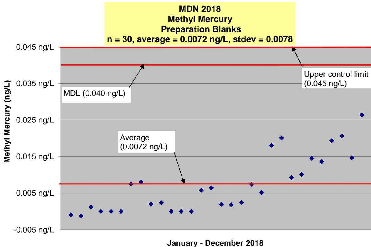
**Figure 4 - Methyl Mercury Concentrations in Reagent Preparation Blanks, 2018**
