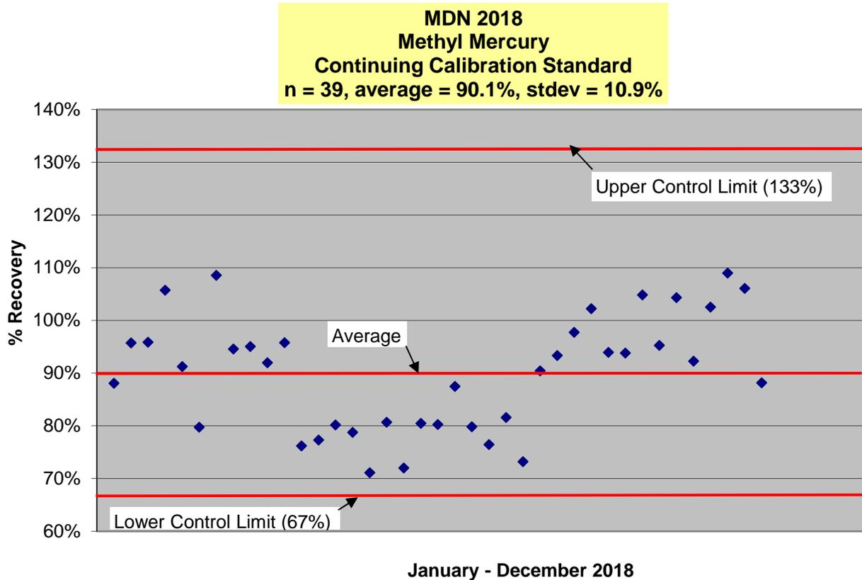
**Figure 6 - Methyl Mercury Continuing Calibration Standard Percent Recovery, 2018**
