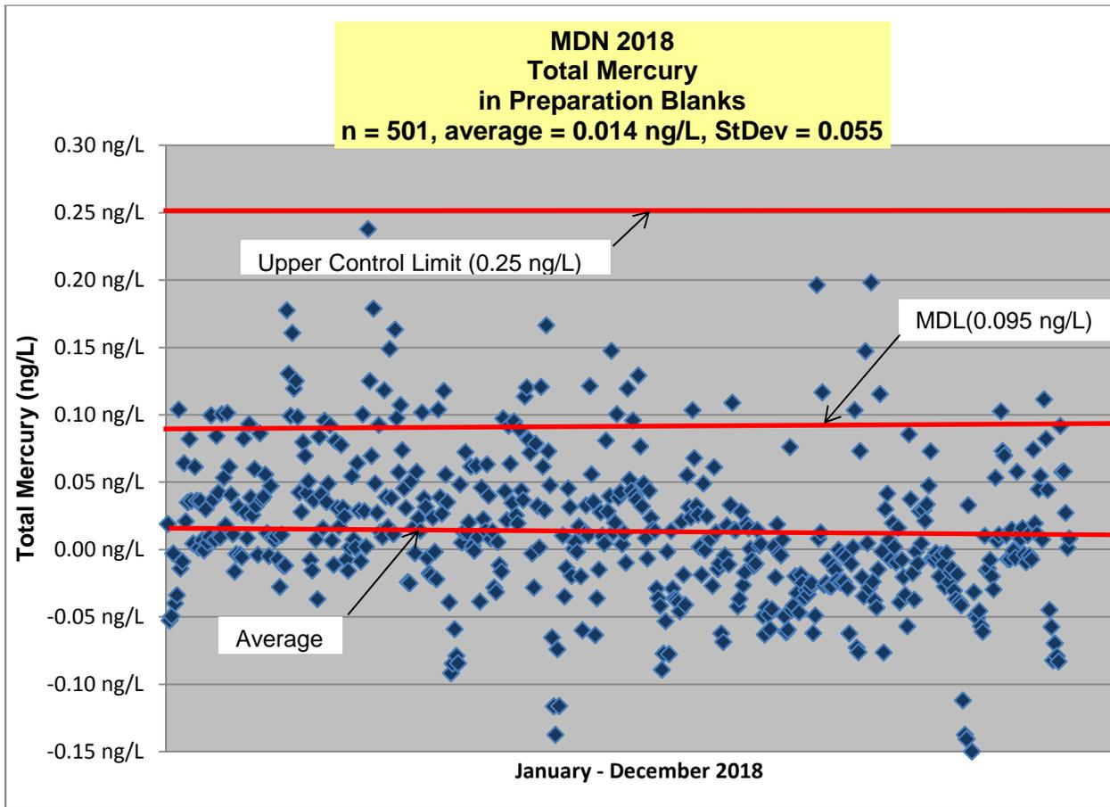
**Figure 3 - Total Mercury Concentrations in Reagent Preparation Blanks, 2018**
