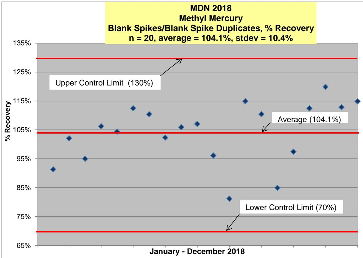
**Figure 16 - Methyl Mercury Percent Recovery in Blank Spikes/Blank Spike Duplicate Samples, 2018**
