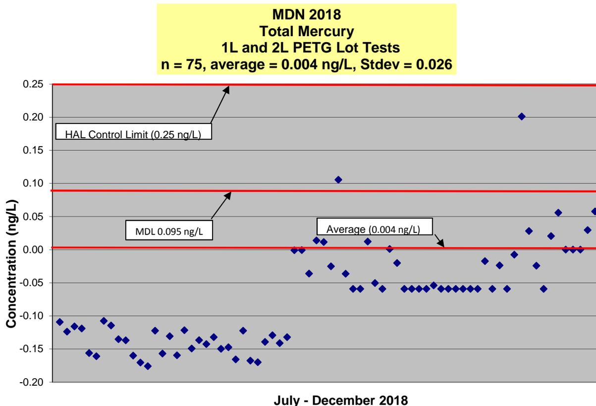
**Figure 2' – Laboratory 1L/2L PETG Lot Tests for 75 Samples in 5 Lots, 2018**
