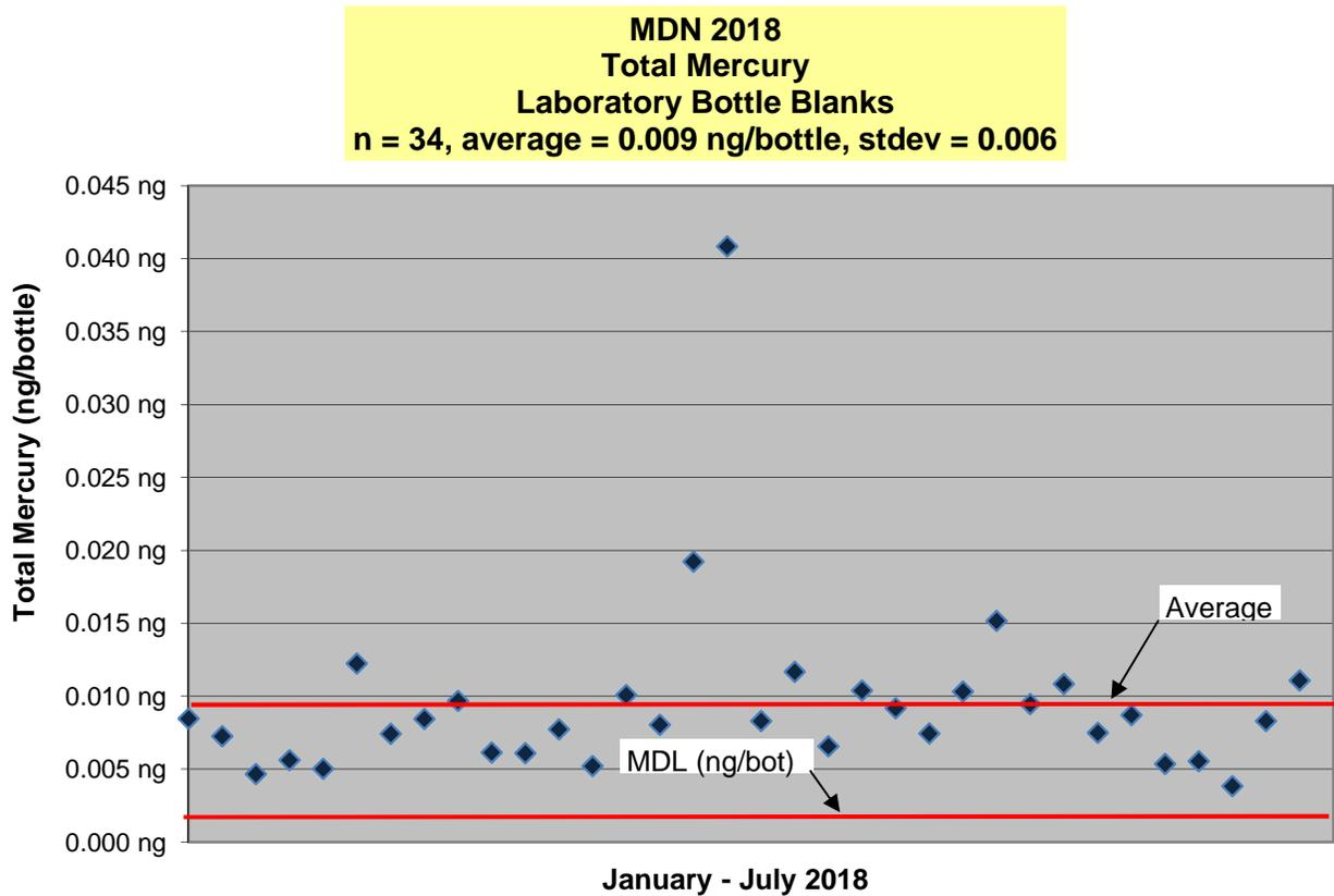
**Figure 1 - Total Mercury Mass in Laboratory Bottle Blanks for 34 Samples, 2018**
