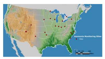
monitoring network for ammonia gas across the Midwest. The goal is to develop, deploy, and operate a costefficient *passive* sampling network for basic ammonia gas concentrations. These two-week integrated values will be used to quantify the spatial and temporal differences in atmospheric ammonia concentrations. The network includes an appropriate quality-assurance program to
