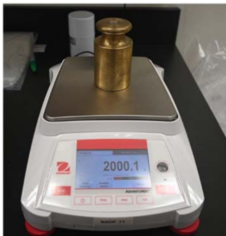
Figure 1. Check balance with calibration weight.
