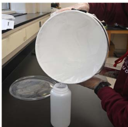
Figure 6. Decant the sample into the sample bottle.
