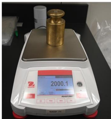
Figure 1. Check balance with calibration weight.
