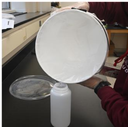
Figure 6. Decant the sample into the sample bottle.
