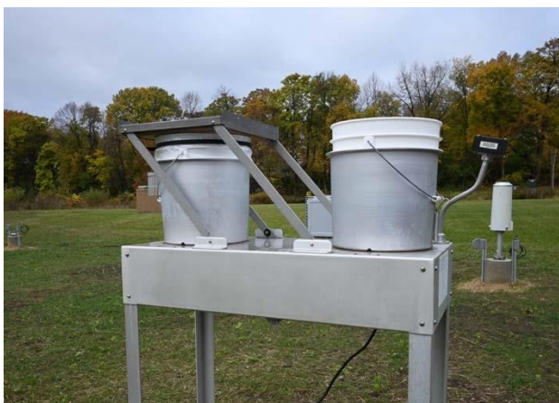
Figure 1. Aerochem NTN bucket collector
