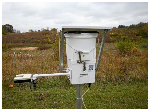
Figure 2. N-CON NTN bucket collector
