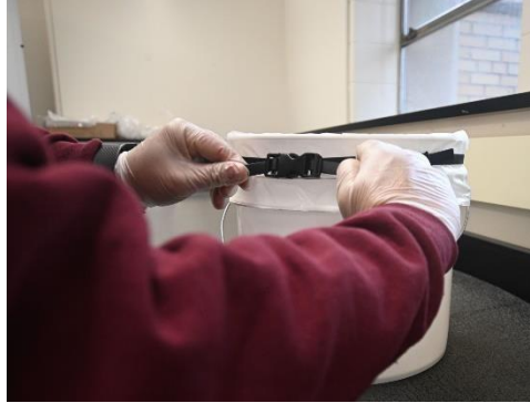
Figure 5. Wrap strap around NTN bucket and cinch to secure the sample bag.
