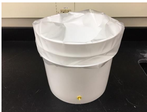
Figure 4. Drape excess sample bag over edge of NTN bucket.
