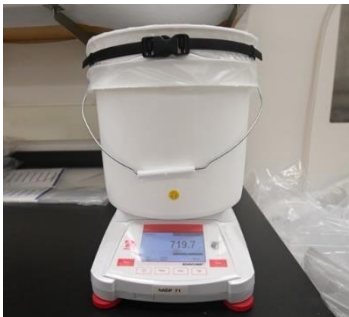
Figure 9. Weigh NTN bucket, sample bag, bucket strap and bucket plug
