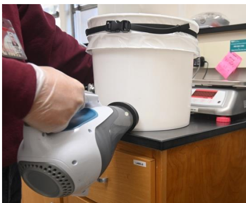
Figure 6. Apply the vacuum to pull the sample bag to the walls of the NTN bucket.
