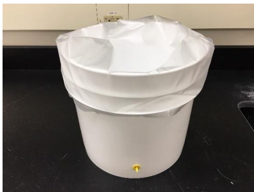
Figure 4. Drape excess sample bag over edge of NTN bucket.
