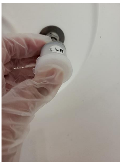
Figure 13. Embossed lid replaced on sampler
