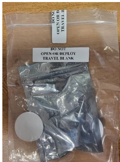
Figure 7. Travel Blank with citric acid filter paper. (leave in sealed bag in shipping box)
