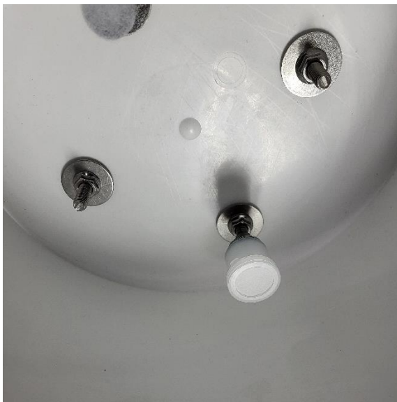
Figure 10. AMoN sampler deployed in shelter.
