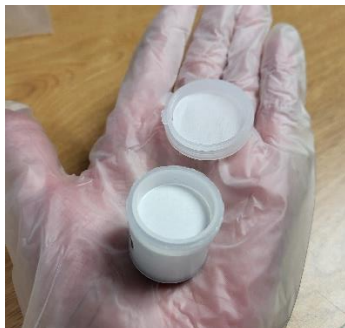
Figure 16. Sampler with embossed lid and PTFE membrane cap removed
