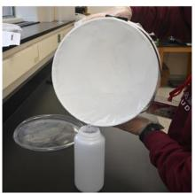
**Figure 6.** Decant the sample into the sample bottle.
