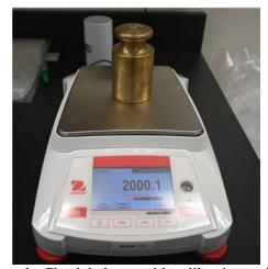
Figure 1. Check balance with calibration weight.
