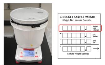
Figure 2. Weigh bucket, bag, strap, plug, and lid.
