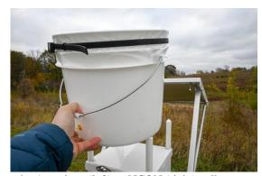
Figure 11. Place the new sample bag bucket on the Aerochem (left) or NCON (right) collector.
