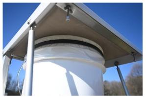
Figure 12. Check the lid pad seal on the sample bag bucket. Aerochem (left) and NCON (right).
