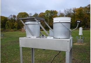
Figure 1. Aerochem NTN bucket collector
