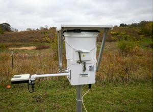
Figure 2. N-CON NTN bucket collector
