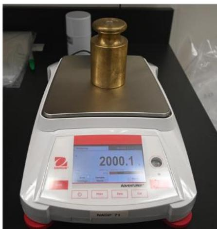
**Figure 1.** Check balance with calibration weight.
