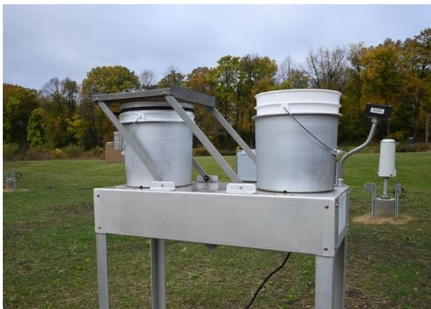
Figure 1. Aerochem NTN bucket collector
