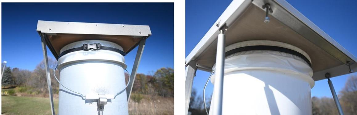
**Figure 12.** Check the lid pad seal on the sample bag bucket. Aerochem (left) and NCON (right).
