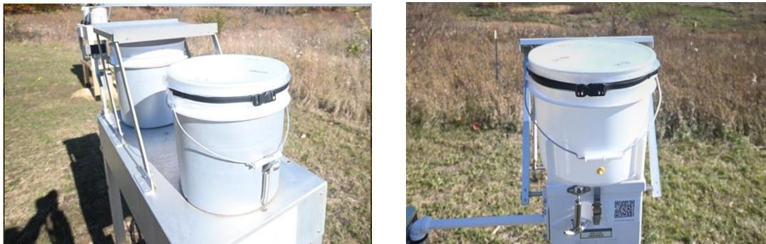
**Figure 6.** Seal the previous weeks sample bag bucket. Aerochem (left) and NCON (right).
