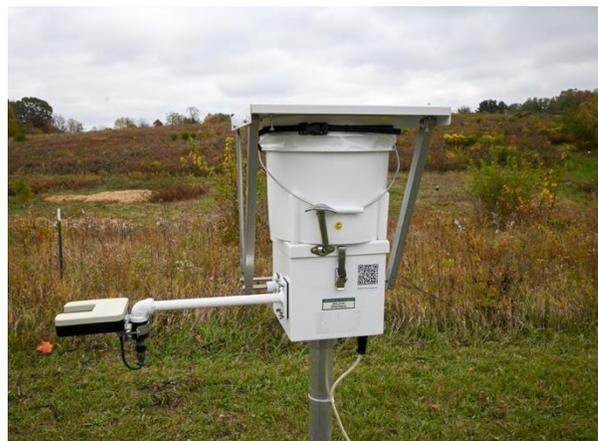
Figure 2. N-CON NTN bucket collector
