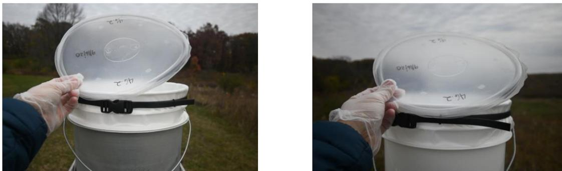
**Figure 5.** Placing the spare lid on current sample bag bucket.
